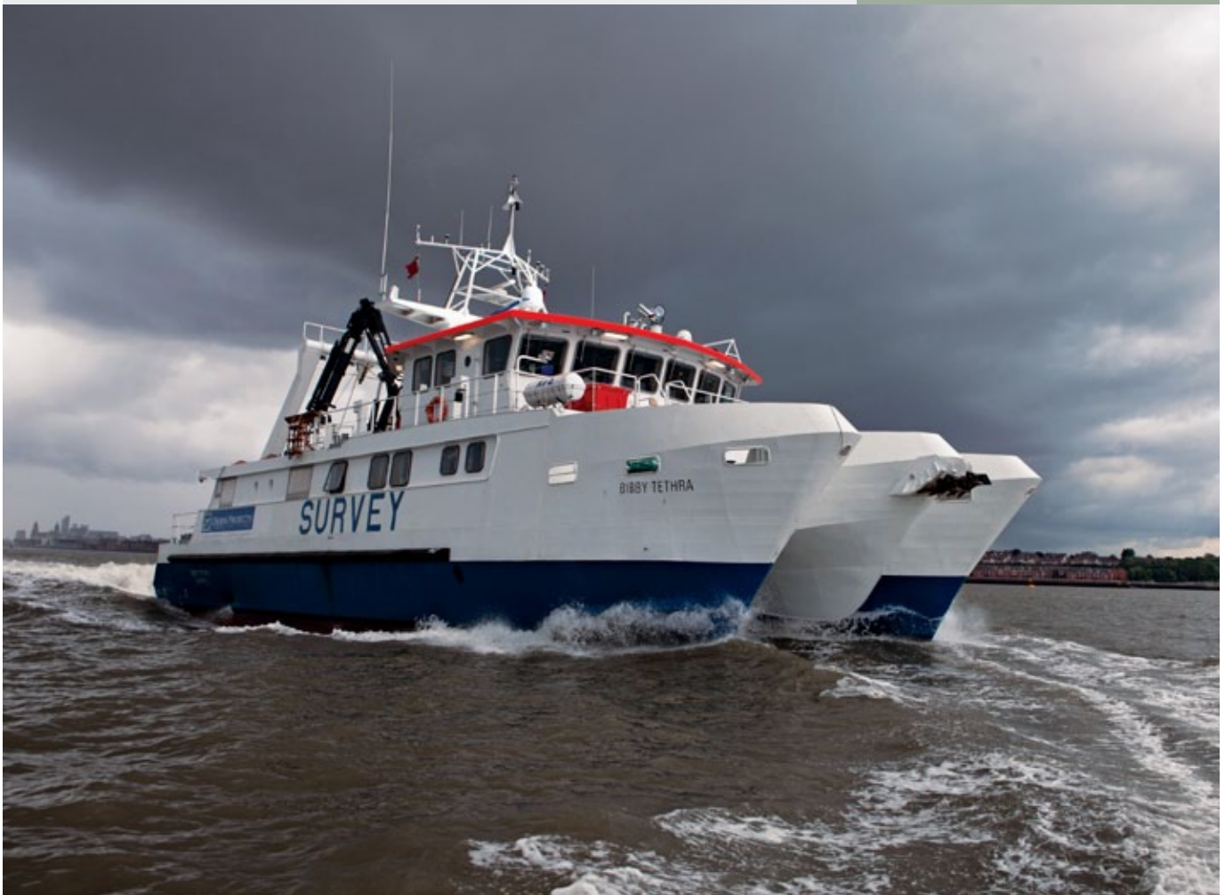
Below and left: SV Bibby Tethra, a 91-foot (28-meter) purpose-built semi-SWATH coastal survey vessel doing seabed mapping for the company Osiris Projects, is the first dynamic positioning boat in Europe equipped with a Twin Disc QuickShift® transmission system, including twin MGX-516DC transmissions and EC300DP electronic controls, driven by Cummins 660-hp (492-kW) engines. The boat will be dedicated to underwater surveys for installation of offshore wind farms in Northern Europe.
