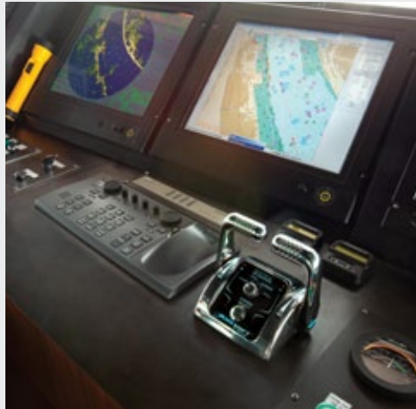
Below and left: SV Bibby Tethra, a 91-foot (28-meter) purpose-built semi-SWATH coastal survey vessel doing seabed mapping for the company Osiris Projects, is the first dynamic positioning boat in Europe equipped with a Twin Disc QuickShift® transmission system, including twin MGX-516DC transmissions and EC300DP electronic controls, driven by Cummins 660-hp (492-kW) engines. The boat will be dedicated to underwater surveys for installation of offshore wind farms in Northern Europe.
