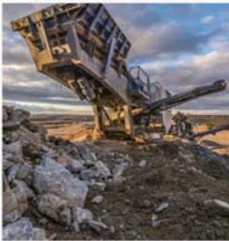
Construction: Rock Crusher
