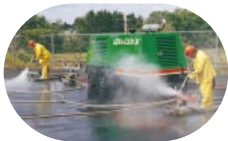
NLB Corporation's Ultra-Clean 36° ultra high pressure pumping unit uses a Twin Disc SP211HP3 PTO to apply 36,000 psi of water pressure to cleaning operations.
