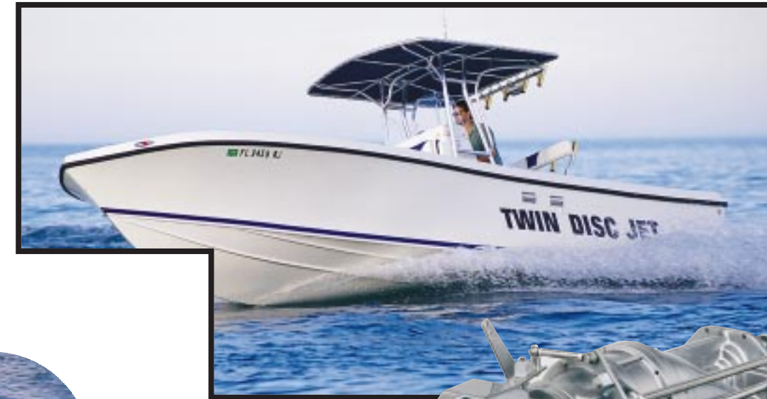
To fully demonstrate the speed, maneuverability and safety of a waterjet, the Twin Disc Propulsion Group equipped this nimble 28' hull with a Twin Disc TDJ110 Waterjet driven by a Yanmar 350 hp engine driving through an MG-507-1 Marine Transmission controlled by an EC-200WJ Electronic Control.
