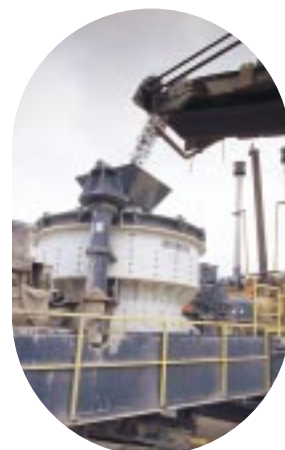
This R.E. Clancy Verticle Shaft Impactor uses a rugged Twin Disc Inline SP318IL PTO to crush limestone in a northern Michigan quarry.
