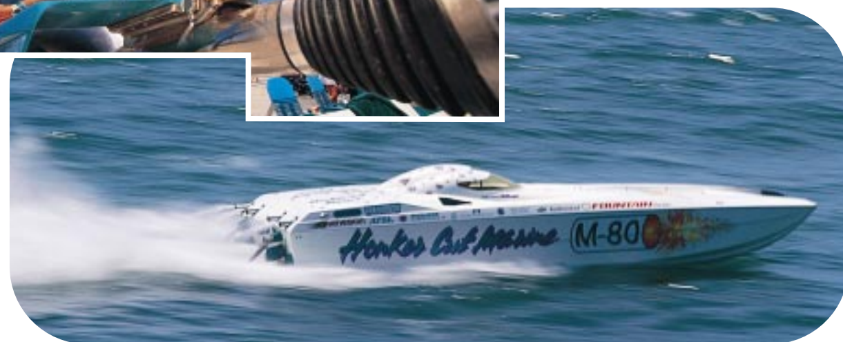
Honker Cut Marine out of San Diego is showing some decisive wins on the American Power Boat Association circuit with its specially prepared 38' offshore boat equipped with twin 920 hp, 510 cubic inch Oldsmobile engines driving ASD 8 Arneson Surface Drives.
