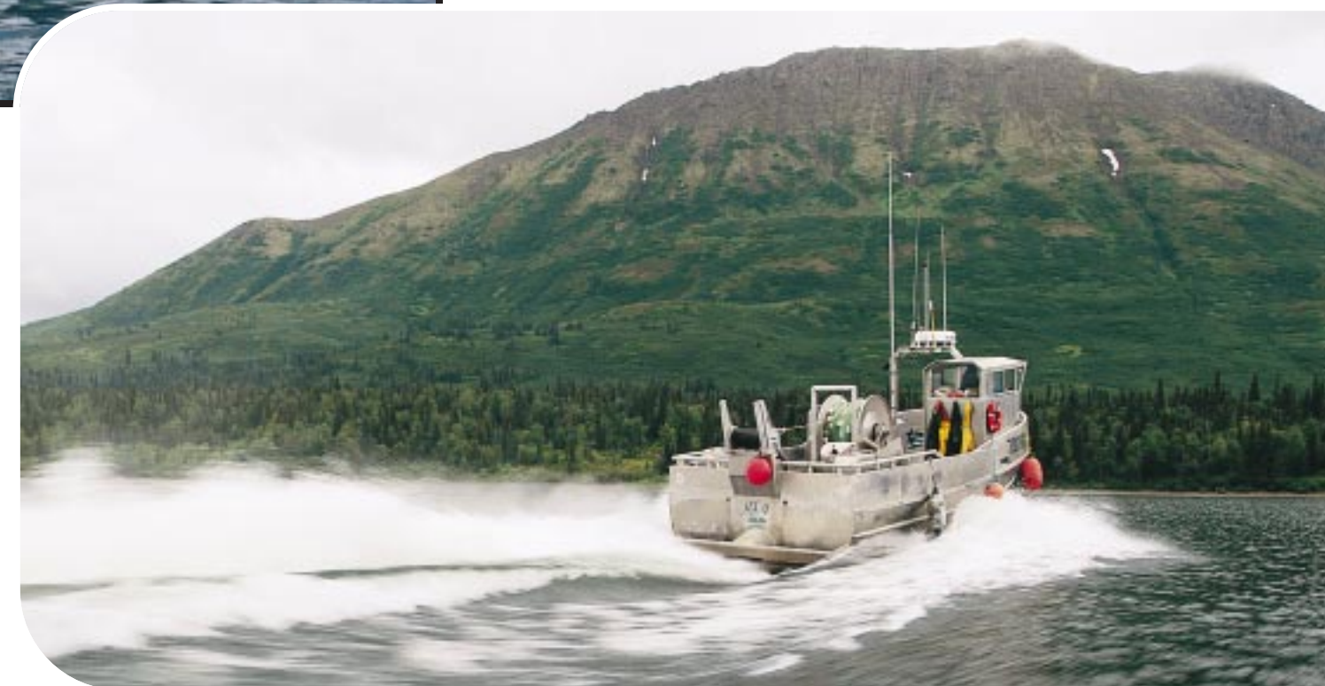
The Ulu , a 32' all-aluminum Bristol Bay Gillnetter made by Stambaugh has the advantage of speed, maneuverability, precise control and no propeller to snag nets, thanks to a Twin Disc TDJ130 Waterjet powered by a Luger 425 diesel and controlled by a two-station Twin Disc EC-200 Marine Electronic Control System.
