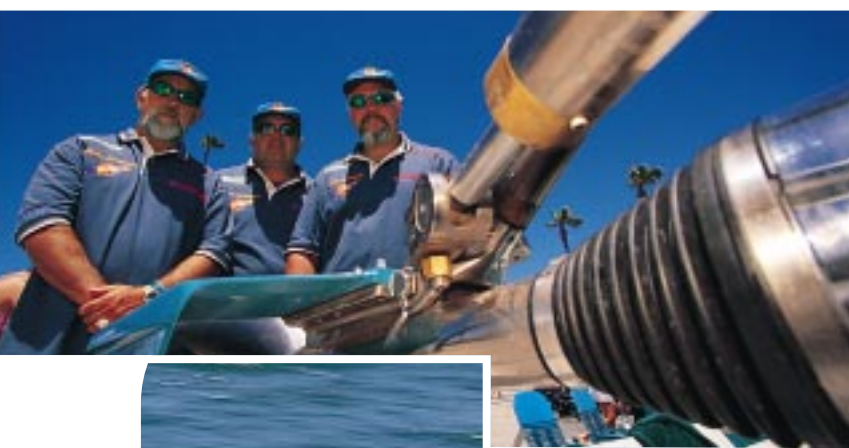
Honker Cut Marine out of San Diego is showing some decisive wins on the American Power Boat Association circuit with its specially prepared 38' offshore boat equipped with twin 920 hp, 510 cubic inch Oldsmobile engines driving ASD 8 Arneson Surface Drives.
