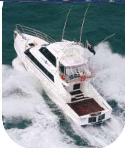
Radar Blue , a 62' Salthouse charter gamefish yacht built in Auckland, New Zealand, is a marvel of luxury and technology. It's powered by twin 660 hp Caterpillar engines driving through Twin Disc MG-5114A Marine Transmissions via Twin Disc EC-200 with three-station electronic controls.
