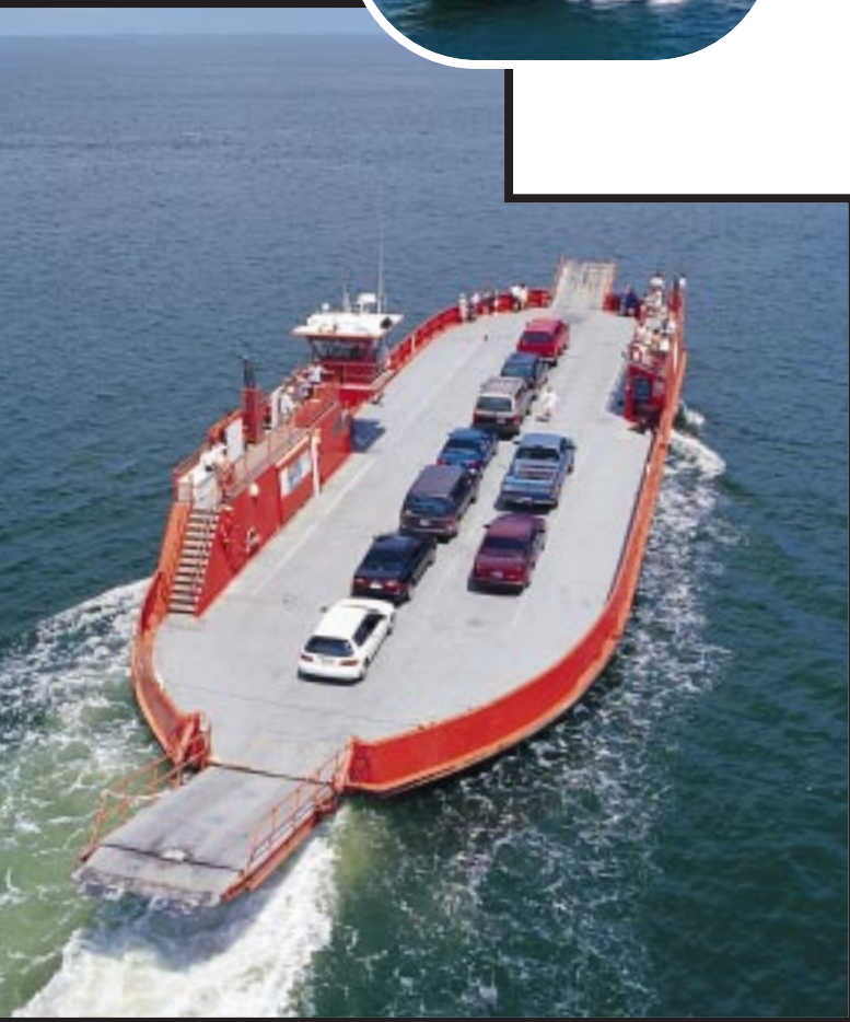
The Ft. Morgan Ferry makes the 4-mile trip across the mouth of Mobile Bay between Dolphin Island and Ft. Morgan, Alabama, sixteen times a day. It uses two Detroit Diesel 12V71 360 hp engines and two Twin Disc MG-514 Marine Transmissions, one set each mounted fore and aft, to push and pull the boat simultaneously.
