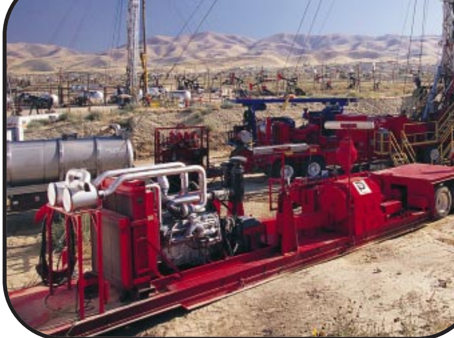
Pool Energy Services facilitates drilling California oil wells with this portable high pressure mud pump driven by a General Engine power package consisting of a Detroit Diesel 700 hp 1292 DDEC engine working through a Twin Disc TD-51-2000 Transmission with Type-8 18" Torque Converter.
