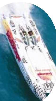
Lanier Racing is turning heads on the Super Boat Association offshore racing circuit with its 41' super unlimited catamaran hulls powered by twin Eickert 960 hp engines driving Arneson ASD 8 Surface Drives to speeds of 130 mph.
