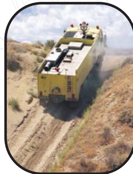
Fully loaded with nearly 3,000 gallons of water, the 30-plus ton vehicle can climb a 40% grade in soft dirt.
