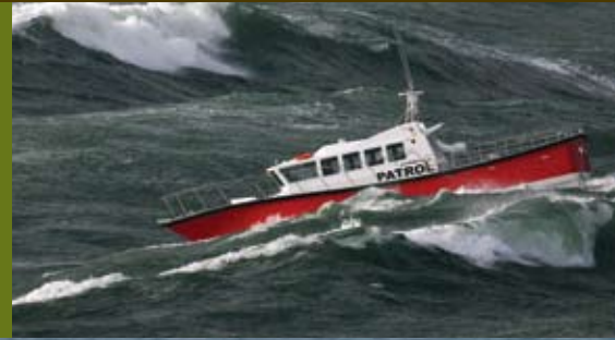
Above: Angus Cambell's Interceptor 55 Orca II, built by Safehaven Marine, County Cork, Ireland, and equipped with twin Scania 650-horsepower (485-kW) engines working through Twin Disc MGX-5114 QuickShift® marine transmissions and EC300 electronic controls, transports passengers and light cargo from home port on The Isle of Harris, 50 nautical miles offshore, to St. Kilda, a wildlife and marine life habitat 45 miles further straight out into the North Atlantic.
