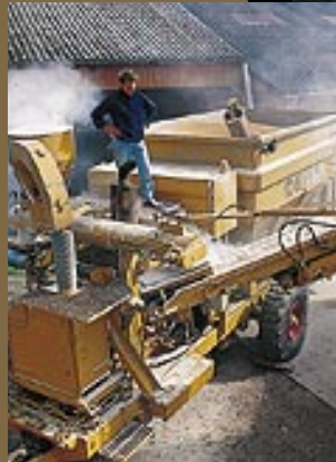
A Twin Disc PTO actuates a mobile corn mill in Aalter, Belgium.
