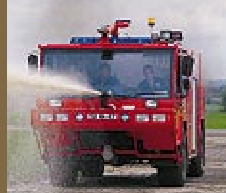
A Simon Access Crash-Fire-Rescue (CFR) vehicle equipped with a 6V-92 DDC 475 horsepower engine and a Twin Disc TD-61-1175 Automatic Transmission System performs a "pump and roll" test run at Staverton Airport in Gloucester, England.
