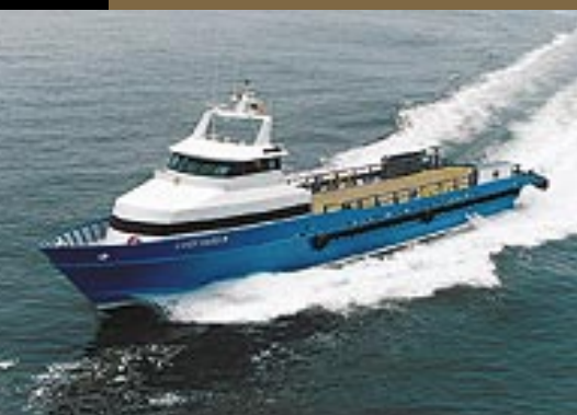
The Swiftships-built 145' Candy Dancer is one of many Diamond Services crew/supply boats working the offshore rigs in the Gulf of Mexico. It has four Cummins turbocharged and aftercooled engines, rated at 700 horsepower, driving through Twin Disc MG-5202 Marine Transmissions.
