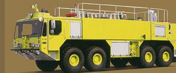
Emergency One's Titan HPR™ 8x8 with its 1000 hp Detroit Diesel engine and Twin Disc TD-61-1175 automatic transmission system can carry up to 4,227 gallons of water and 405 gallons of foam concentrate and still achieve 50 mph in under 30 seconds.
