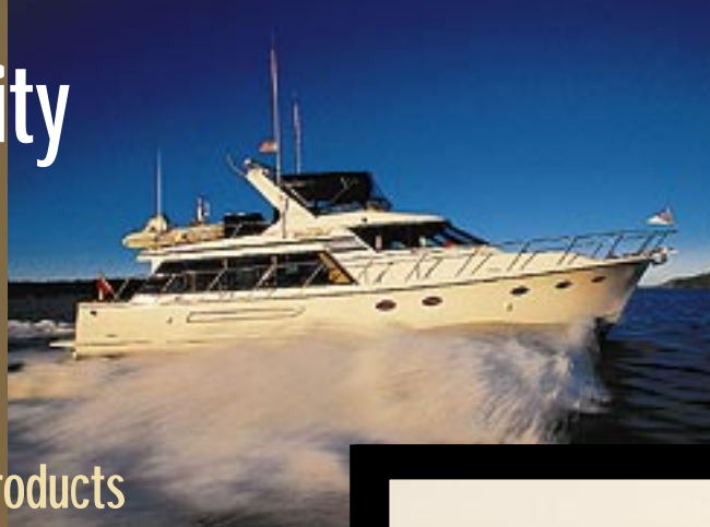
Off the San Juan Islands, the Ocean Alexander 52' Windstar easily makes way with its twin Detroit Diesel engines generating 400 horsepower each through Twin Disc MG-507-1 Marine Transmissions.
