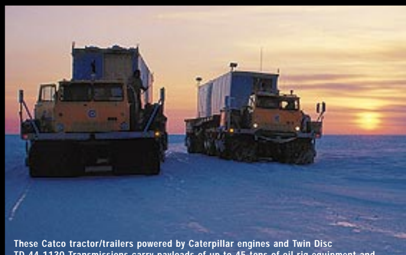
The unique propulsion system includes low pressure tires driven by outside-wheel drive arms.
