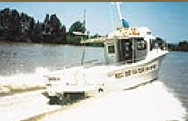
This 36' Stebercraft dive boat with a Cummins turbo-charged diesel engine connected to a TDJ130 Waterjet has the power and maneuverability to navigate the difficult and shallow Wooli River to quickly reach dive sites off New South Wales, Australia.
